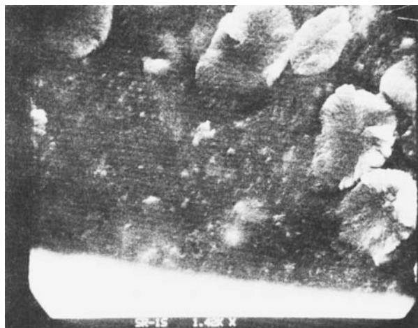
Figure 4 —Insulin adsorbed onto silicone rubber under high shear, 1600 \times .
