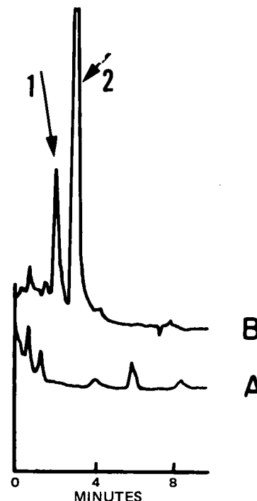
Figure 1 —Chromatogram of the extract of a 1-ml plasma blank (A) and plasma with 25 ng/ml of diphenhydramine and 100 ng of orphenadrine added (B). Key: (1) diphenhydramine; (2) orphenadrine.
